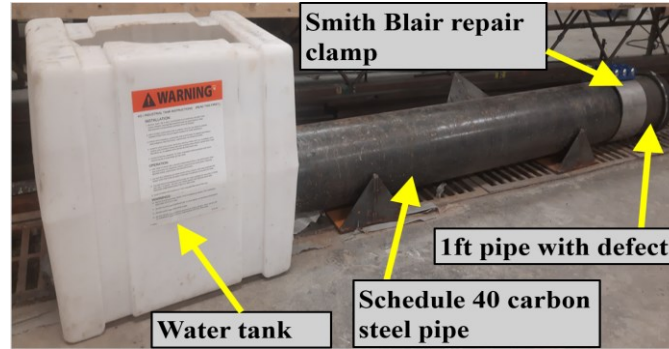
Figure 3. Lab test set-up with 8-in-diameter schedule 40 pipe with various defects.
